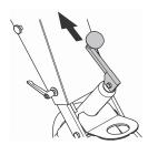
Carefully fold the machine forward. Put padding between the motor and the electric box to prevent damage to the machine.
