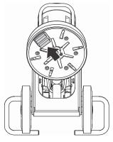
Once new diamond segments have been attached, reverse procedure to lower machine to ground.
