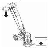
Press the start button and keep it pressed a few seconds to start the machine.
